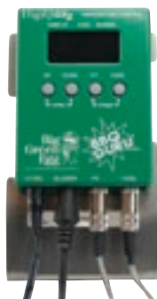
Left: The BBQ Guru DigiQ System automatically controls the internal temperature of the EGG.
